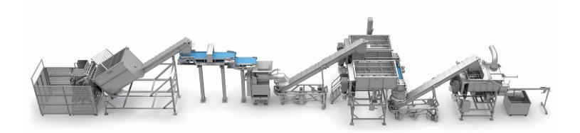
Pre-Blending offers a seamless, accurate solution, but the equipment costs, added footprint size, maintenance, and sanitation requirements must also be considered. In this method, lean and fat are transferred into one of two pre-Blenders. The goal is to create a homogeneous batch of each lean point (preground) from which the final Mixer can draw.
